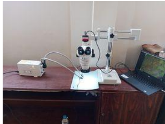
Fig 1: Examine coin under stereomicroscope
